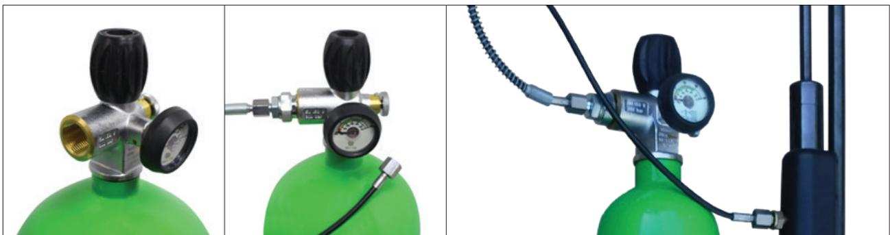
To fill a PCP air rifle, attach the hose provided to the cylinder and the PCP air rifle, slowly open the cylinder valve by rotating it anti-clockwise (half a turn may be sufficient), fill to 200 PSI below the recommended air rifle fill pressure, turn off cylinder valve and repeat this process to full service pressure 30 minutes later. This two stage filling process enables the air in the air rifle to stabilise and ensures that it is not accidentally over-filled.
